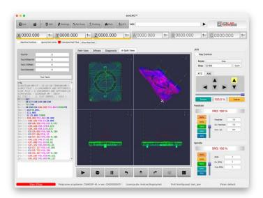
The program uses the popular, standard ISO G-Code trajectory description language, but when loading and working it analyzes every segment, arc or corner and practically recreates all shapes using advanced mathematical algorithms. Many variables are taken into account, such as given tolerance, speed, accelerations and type of curvature to generate data for the controller and axis drives in such a way that the movement is accurate, smooth and fast.
